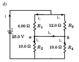
I<sub>s</sub> is the current through the switch  $I_1 = I_s + I_2$  $I_s = I_1 - I_2 = 2.34A - 1.56A = 0.78A$
