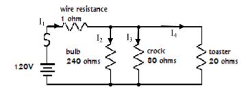
The light bulb, the toaster and the crock are in parallel; we can find the equivalent resistance:  $R_{eq} = (R_{bulb}^{-1} + R_{crock}^{-1} + R_{toaster}^{-1})^{-1} = (240^{-1} + 80^{-1} + 20^{-1})^{-1} = 15\Omega$
